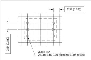
Holes may be omitted for variants with fewer than 6 pins. Unless otherwise stated all dimensions in mm (inches)  $\pm 0.25$  (0.01). All pins on a 2.54 (0.1) pitch and within  $\pm 0.25$  (0.01) of true position.
